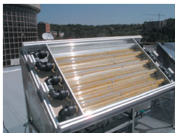
Photochemical reactions are used increasingly in “green” technology. This reactor on the roof of Complutense University of Madrid is used for water disinfection. A polymer-supported dye absorbs sunlight to convert oxygen to a more reactive state (“singlet oxygen”), which destroys harmful bacteria in water (picture courtesy of Professor Guillermo Orellana, UCM).
