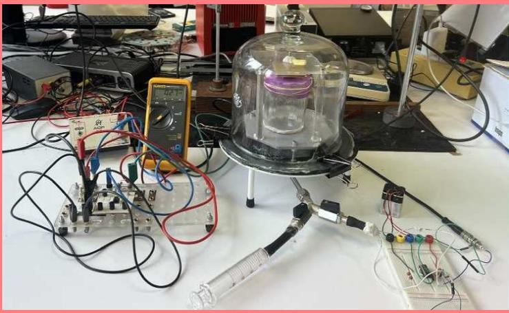
The photograph shows a laboratory setup for measuring pressure. It includes a glass bell jar on a stand, a multimeter, and various electronic components and wires connected to a circuit board.
