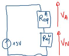
$$V_A = \frac{15/R_{eq}^N}{1/R_{eq}^N + 1/R_{eq}^A} = \frac{15}{1 + \frac{R_{eq}^N}{R_{eq}^A}} = 6,7 \text{ V}$$
